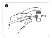
Then, unscrew and remove the small compression nut from the diverter valve. Slide the nut over one end of the white inlet hose. Make sure the threads are positioned so it will screw onto the diverter. Push the hose firmly onto the nipple, then screw the compression nut back on.
